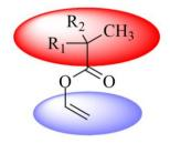
Both  $R_1$  and  $R_2$  are alkyl with total 7 carbon atoms. The tertiary carbon structure has large steric hindrance, which is similar to umbrella structure. Therefore, it has good hydrophobicity, acid and alkali resistance, and UV resistance. Vinyl is easy to copolymerized with acrylics, vinyl acetate and other monomers for binary, ternary and multicomponent to form a copolymer tertiary carbon emulsion.
